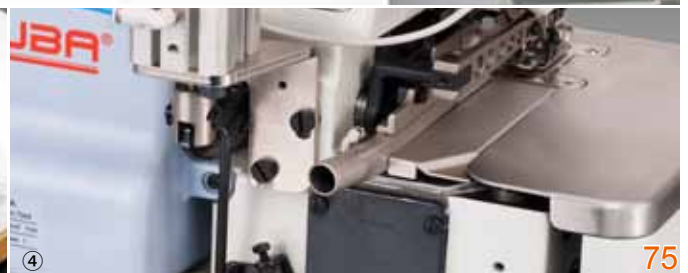
上图仅为缝纫机, 气阀, 风管, 集尘袋之相对位置示意说明, 实际使用上建议机械阀搭配离合器马达 The above example is for the purpose of position explaining between machine, air switch, air hose, and dust bag. Practically the mechanical type air switch is mainly suitable for clutch motor.
